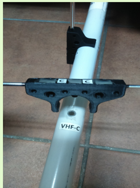
Fig. 5: Detail of the element support with its positioner protrusion.
