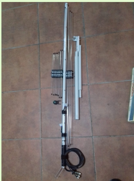
Fig. 4: View of the antenna with all disassembled elements.
