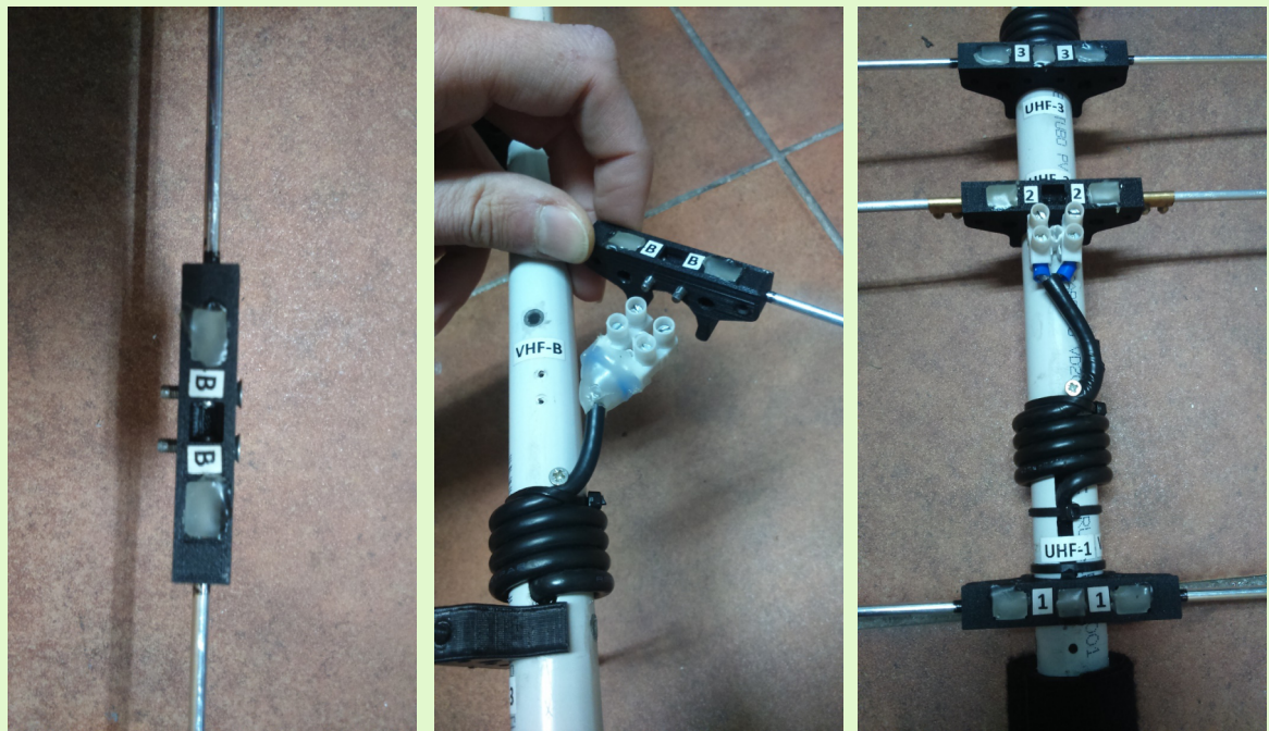
Fig. 6: Detail of the dipole feeding line.
