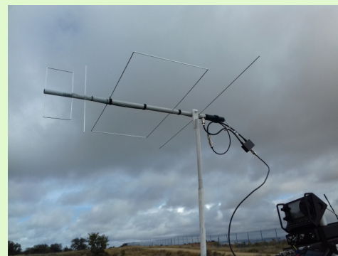
Fig. 1: IOio antenna, design by EA1CYQ – Juan Antonio, ready for the portable operation as a handheld antenna..
