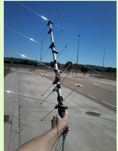
Fig. 2: The photograph of the "PArrow" shows the settings. Actually consists on two DK7ZB antennas placed in perpendicular on a single boom.
